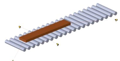
Slab Length - Width measurement using 4 Laser Sensors Dilas FT.
